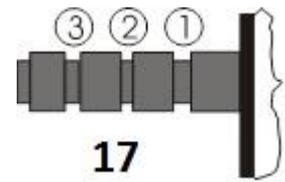
Slip the loop of the anti-skating weight's thread over the second groove of the stub to set the correct anti-skating force for the factory-fitted cartridge. Feed the thread through the loop of the wire support (15).
